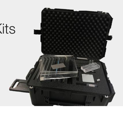
Criteria for acceptance testing of 3D Tomosynthesis Mammography systems has been internationally defined by the IEC, per protocol 61223-3-6. To fulfill these tests, a variety of tools are required, some of which are unique to Digital Breast Tomosythesis (DBT).
