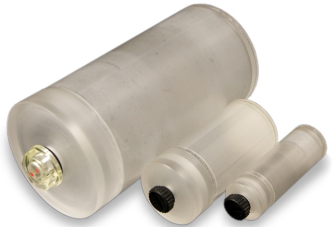
Standard versions (Ø 20, 32 and 60 mm) of the QRM Micro-CT Water Phantom
