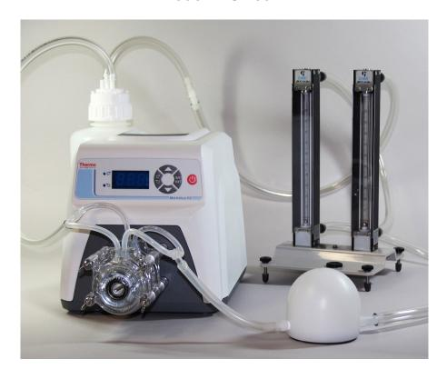
The Model 700-D, Doppler Flow Digital Controller and Pumping System, combined with an ATS Doppler Flow phantom provide an easy and accurate means of evaluating an ultrasound Doppler imaging system's ability to detect sensitivity at varying depths, maximum penetration, flow velocity, location and directional discrimination.
