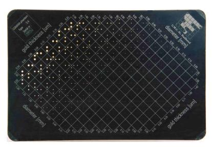
detecting very low contrast and detecting very small details. With the phantom the "threshold contrast" as a function of the object diameter can be determined and plotted in a Contrast-Detail curve.
