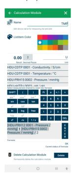
The formulas for the calculations can be easily edited and allow the insertion of measurement channels and any mathematical expressions.
