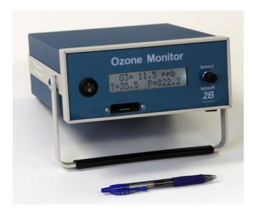
The 2B Technologies Model 202 Ozone Monitor™ is designed to enable accurate and precise measurements of ozone ranging from low ppb (precision of ~1.5 ppb) up to 250,000 ppb (250 ppm) based on the well-established technique of absorption of UV light at 254 nm. The Model 202 Ozone Monitor™ is lightweight (5.5 lb, 2.5 kg) and has a low power consumption (12V DC, 0.60 amp, ~7.2 watt) relative to conventional instruments and is therefore well suited for applications such as:
