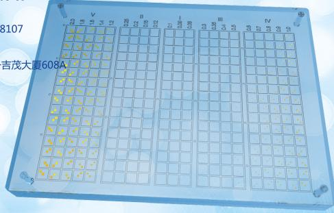
Upgraded contrast details mammography phantom according to European Protocol for quality assurance in Digital Mammography. It may be used to determine if mammographic images indicate objects with very low contrast and very small diameter, to find out the optimum exposure technique, or to compare image quality at various object thicknesses by variation of the amount of PMMA thickness.
