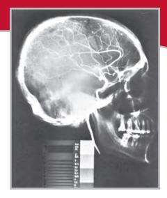
The ANGIOGRAPHIC HEAD PHANTOM provides a "dry run" to completely check out angiographic equipment and ensure that is operating satisfactorily in all significant details before subjecting patients to radiological procedures. If the imaging system malfunctions, the phantom also plays a critically important role in isolating and verifying correction of the problems. The ANGIOGRAPHIC HEAD PHANTOM confines the variables to components and technique and is an invaluable service and teaching tool.
