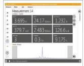
Data parameters selected are displayed after each exposure along with the dose rate waveform
