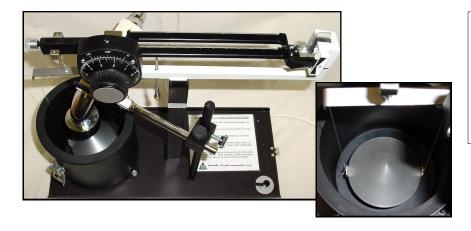
The heart of the UPM-30 unit is its air-filled conical target. The transducer to be tested is center mounted over this conical target with the transducer's radiating area immersed, face down, in the water medium
