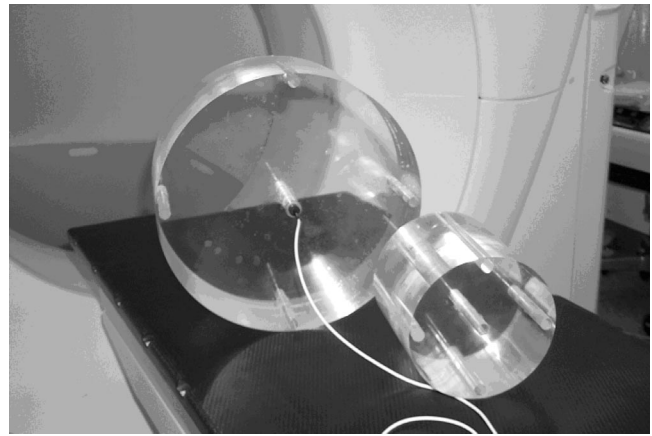
Fig. 7. A body and head phantom for measurement of dose from CT-scans. Pencil ionization chamber is inserted in the center of the body phantom.
