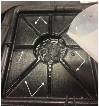
**1c.** Kinks in the tubing will cause pumps to fail. Sometimes old filters can become dislodged and clog the pumps as well. If the pump is clear of obvious defect, begin filling the pump reservoir with water. Be sure to fill until the channels at the top of the reservoir are full.
