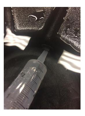
**3c.** If these ports do not being flowing, there may be a kink or issue with the pump filter or possibly trapped air. To deal with potentially trapped air, you can fill a clean 60cc syringe with water and use it to push water into the 3 intake ports within the pump reservoir. If a flow problem persists, submit the pump to the current pump assembly and maintenance personnel for testing and repair and use a different pump to proceed with your testing.
