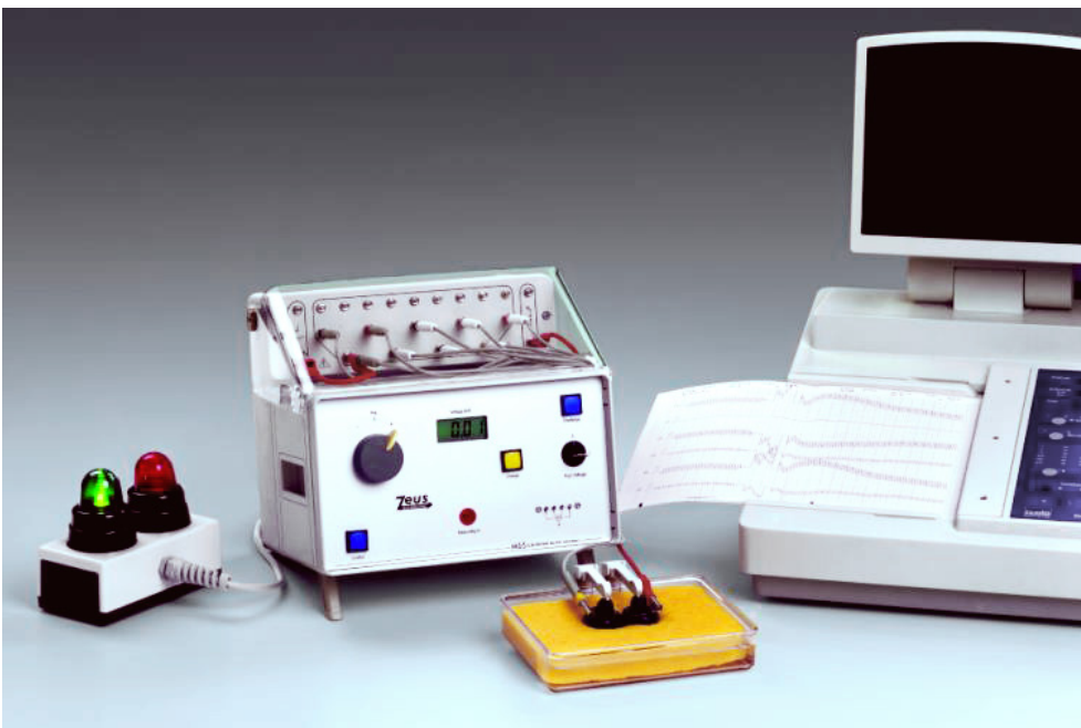
Figure 4-1: Testing the recovery time in response to defibrillation discharge
